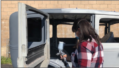
Priming before applying final paint color.
